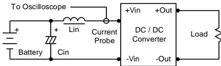
**Peak-to-Peak Output Noise Measurement Test**
