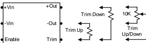
A 10K, 1 or 10 Turn trimpot is usually specified for continuous trimming. Trim pin may be safely left floating if it is not used.
